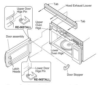
Figure C-2. Door Replacement and adjustment
